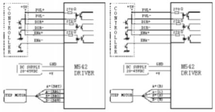
Figure 9: Driver connection in a stepping system
