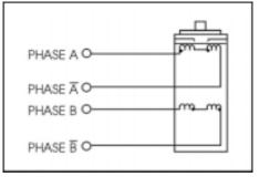
Figure 8: 4 Lead Motor Connections
